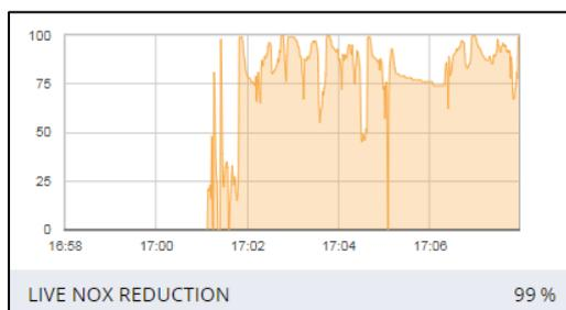
**Example 1:** Exhaust Gas aftertreatment systems are required to stream live nitrogen oxide (NOx) reduction data in compliance with the Transport for London (TfL) NOx abatement programme. By using the AWS IoT protocol, data collected by sensors at the tailpipe are presented on the VPVision web browser reliably within seconds of each reading, providing both a live read out and aggregated performance data.
